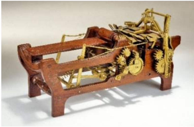
Patent Model for a Paper Bag Machine, 1879.
